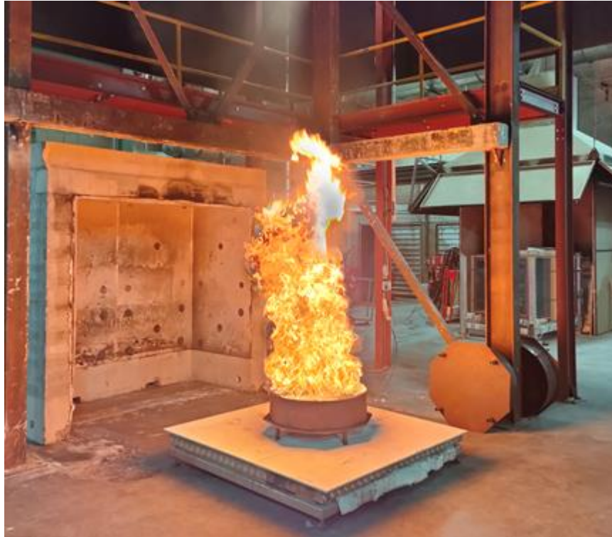
Figure F6. View of the hood calibration with one heptane pan
