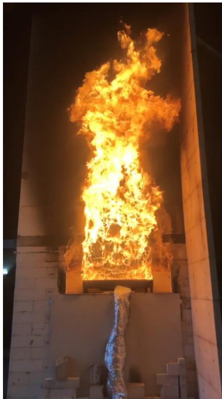
Figure 3.11. Photo from the gas test using 100/80 cm high combustion chamber/opening and a mass flow corresponding to 2.2 MW.
