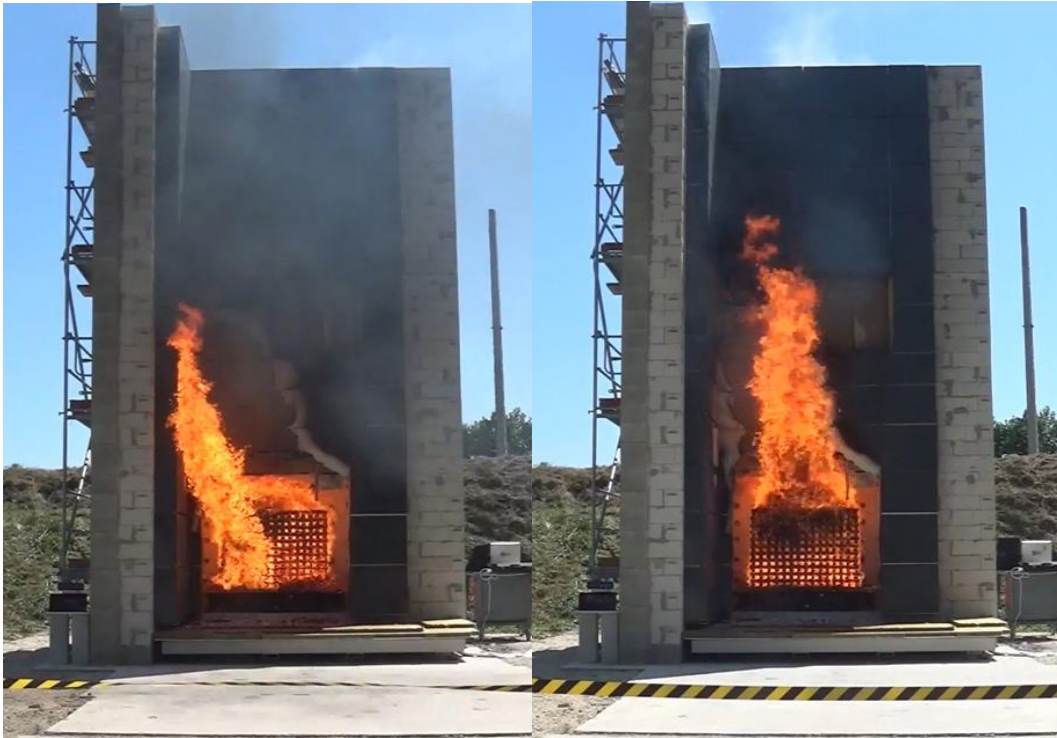
Figure 5.14. Video captures of large-scale test at ÉMI Hungary on EU Aluminium façade at times 21:30 (left) and 22:05 (right) from ignition.
