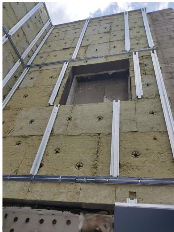
Figure 4.3. Specimen without the aluminium cassette cladding at ÉMI's laboratory.
