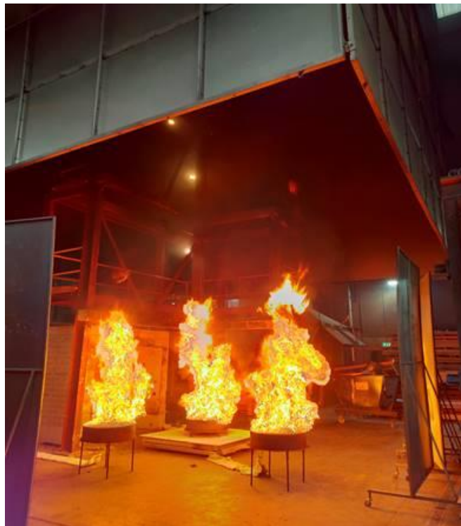
Figure F8. View of the hood calibration with 3 heptane pans
